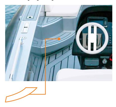
Attach EVA foam boat decking to fiberglass with gelcoat with 3M™ Adhesive Transfer Tape 9775WL
